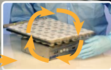
The Dilushaker™ III is an orbital shaker that vortexes each diluent the same way, every time
