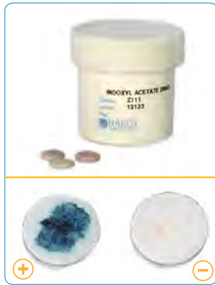
Indoxyl acetate disks, Cat. no. Z111. Showing positive (left disk) and negative (right disk) reactions.
