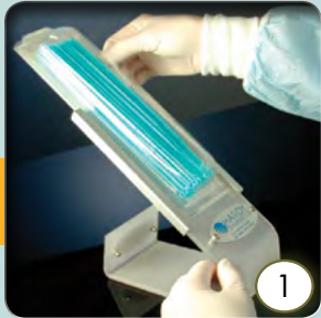
1 Slide resealable loop pouch into LoopCaddy™.
